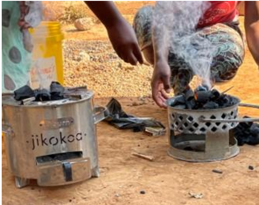
Fuel-efficient cookstove provided by organization (left), and the traditional stove (right)
